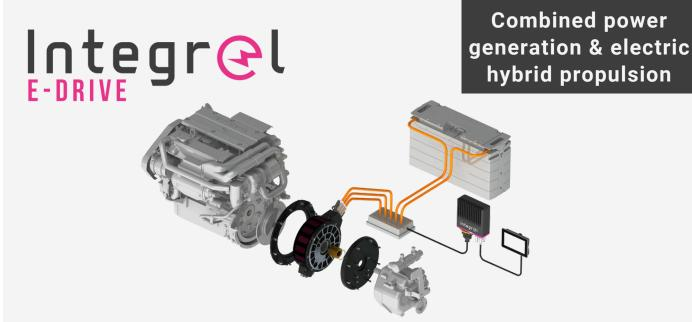
Fitted at the point of manufacture between the engine and gearbox, Integrel E-Drive 15 SE delivers 20 hp of electric propulsion and 15 kW of power generation for single engines and monohulls.
