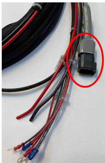
Yanmar Connection on the Controller Loom
