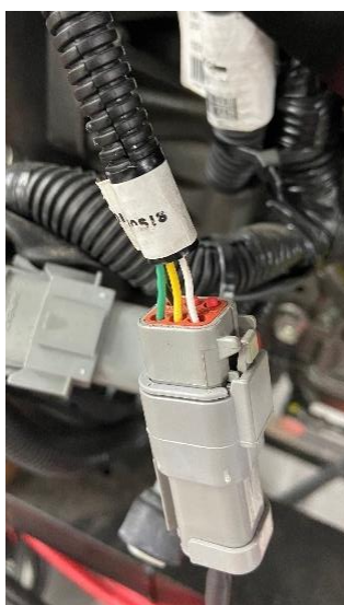
J1939 is labelled as Diagnostic on a Yanmar Engine
