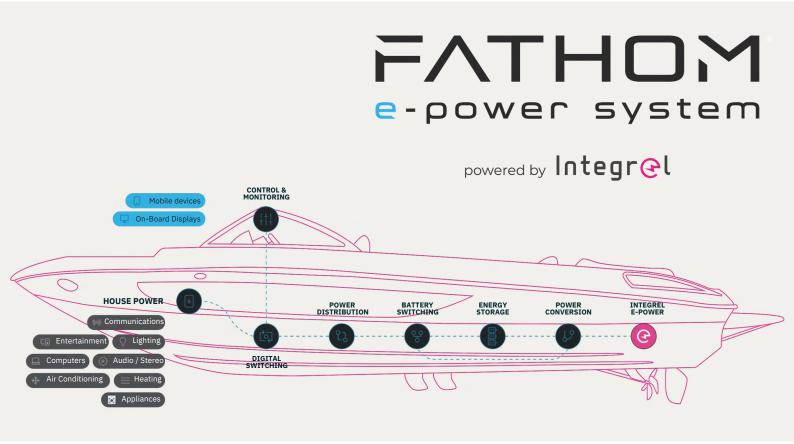
The Integrel E-Power 15/30 integrates seamlessly with the Fathom® e-power system from Navico Group, and delivers unprecedented power generation, intelligently stored in 48V Mastervolt batteries.
