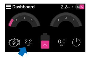
With the port engine running at engine idle, E-Drive generates around 2 kW of power as indicated by the blue arrow in the picture above.
